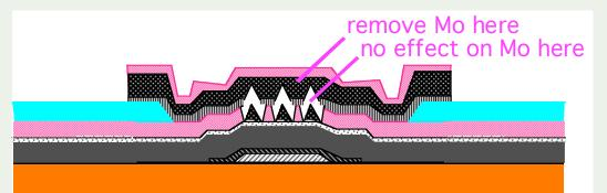
Approach: use electrochemical etch since 'button' is electrically isolated from emitters
